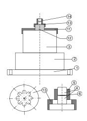
smoothed and the weight with drop and retaining releasing device. The heavy iron block is essential to adsorb shock waves caused by the falling weight. Both guide bars are attached to the column by means of three brackets. The column also carries a toothed rack to arrest
