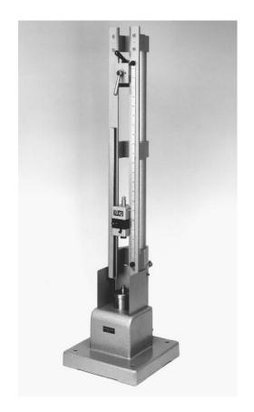
faces  $r_a$ =0.08  $\mu$ m) $\circledast$ , a hollow steel collar (Ø16 mm; height: 13mm; polished bore of  $10^{+0.005}_{+0.010}$ ) $\circledast$  and a centring ring (13) for fixation. The assembly is placed onto a small anvil 26x26mm (12).
